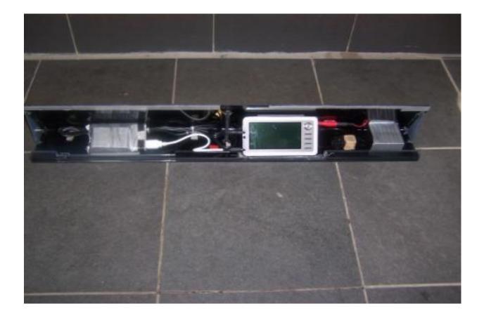
Another example of a PIN capturing device installed on the inner side of the light diffuser fascia piece (above the ATM screen). Can you see the camera?
