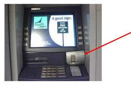
• Top photo shows an unadulterated ATM fascia. The flashing lead through entry indicator is easily observed.
