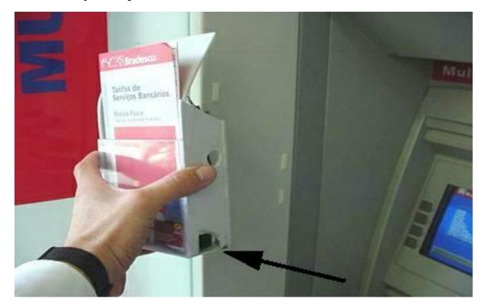
The last area of focus is the ATM keyboard fascia. Offenders are known to place the skimmer plate on top of the existing keyboard.
